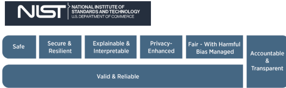
FIGURE 4: CHARACTERISTICS OF TRUSTWORTHY AI SYSTEMS. VALID & RELIABLE IS A NECESSARY CONDITION OF TRUSTWORTHINESS AND IS SHOWN AS THE BASE FOR OTHER TRUSTWORTHINESS CHARACTERISTICS. ACCOUNTABLE & TRANSPARENT IS SHOWN AS A VERTICAL BOX BECAUSE IT RELATES TO ALL OTHER CHARACTERISTICS.
